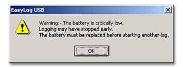
The data logger has stored any readings taken and safely shut itself down. No more readings will be logged and the battery MUST be replaced.
