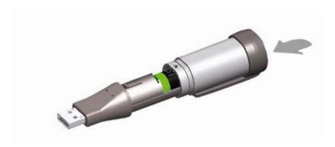
Slide the two parts of the data logger enclosure back together again, until a click is heard. This confirms that the two parts are snapped together correctly.
