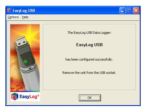
Remove the Data Logger from the computer and place it in the location where you want to measure temperature.
