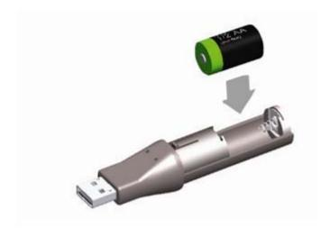
Remove the old battery and dispose of it in accordance with local regulations. Observe warnings on the battery casing.
