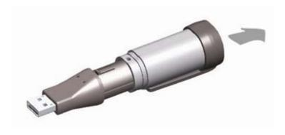
While the tab is pushed down, gently pull apart the two parts of the data logger enclosure.
