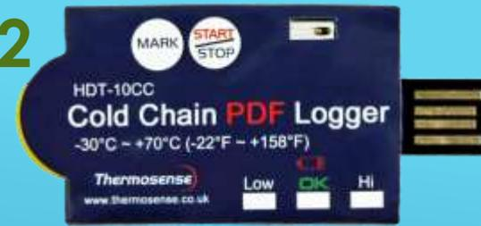
To activate the Logger you have to hold the “START” button for 2 seconds.
