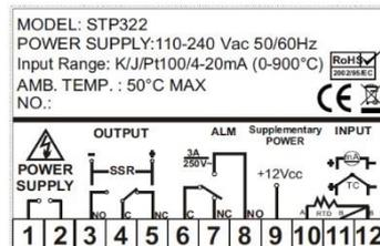
N.B. For 2 wire RTD, white lead 10, red lead 12 and link pin 11 and 12
