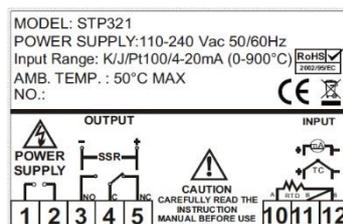
N.B. When using 4-20mA Input, use a precision 250 Ω resistor across terminals 11 and 12 to generate 1-5V input
