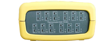
Top view (12 x thermocouple inputs)
